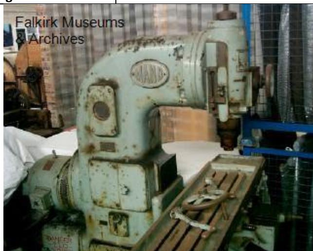
A large, light-green vertical milling machine. The side panel has a circular hole and the word "MANN" stamped on it. The machine is mounted on a heavy base with various adjustment knobs and a worktable. |
