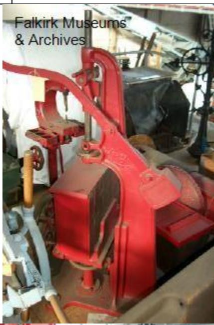
A photograph of a large, red-painted morticing machine. The machine is made of cast iron and has a rectangular base. A prominent red wooden box is attached to the side, containing interchangeable chisel heads. A long wooden lever handle is attached to the side of the machine, with a counterweight at the end. The machine is set against a background of a workshop or museum setting. |
